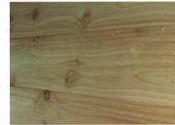
UK grown western red cedar rainscreen boarding.
